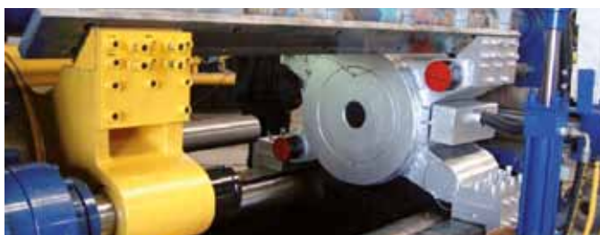
Aluminium extruding press
